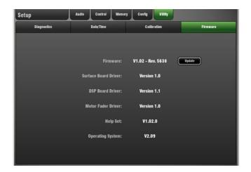
**To check the current Firmware versions** – You can view the GLD Firmware version on the **Home** screen or use the Firmware Setup page to view further details on the system firmware and other drivers within the GLD.
