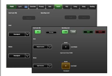
Use the drop-down menus to assign the Insert **Send** and **Return** to physical sockets, the I/O Port or an FX unit. Touch Apply.
