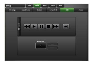
**To change the MIDI Channel** – Touch the MIDI Channel box. Turn the Rotary to select the required channel number. Touch Apply to accept or Cancel to leave unchanged.
