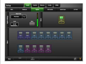
The SigGen routes through the mix master processing, therefore will be affected by the mix EQ and compressor.
