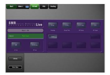
Touch the FX parameter controls and use the screen Rotary to adjust values. Touch a tab at the top of the screen to open the PEQ or routing window. The 4-band PEQ is available within the FX Return strip.
