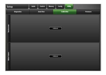
**To calibrate the Touch Screen** – Touch the Calibrate button. As accurately as you can touch the circle at the top left of the screen. Repeat for the other three corners.
