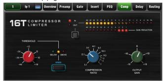
Parallel Path - Lets you mix the dry path 'uncompressed' signal with the compressed output. This 1970's studio technique also known as 'New York compression' is useful in live audio. By mixing the raw signal with heavily compressed material (with make-up gain) low level detail is amplified while the high level transients are preserved from the raw signal.
