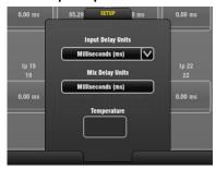
The default delay unit is time in 'ms' (milliseconds) but can be changed to distance in 'metres', 'feet', or to 'samples. This can be changed globally for the Input channels and for the Mix channels. GLD compensates for the effect of temperature on delay. Enter the ambient temperature if distance is chosen.
