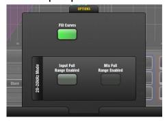
The frequency range for the 4 bands may be set globally for all inputs or mixes to be limited or full **20Hz to 20kHz**.
