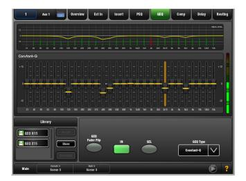
Frequency response curve – The top part of the screen shows the combined response of the slider settings. This can show the response differences between the four GEQ types available.
