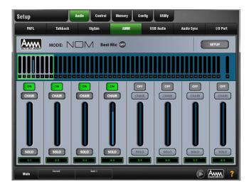
NOM (Number of Open Mics) mode evolved from the AMM developed for the Allen & Heath IDR8 installed sound processor, NOM mode acts as a gate, turning an input on when a threshold is passed. The level adjustment for each open input is equal and depends on the number of microphones open and the NOM attenuation parameter which sets the amount of attenuation applied for every doubling of open microphones.
