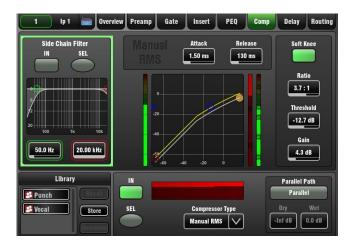
**Ratio** - Sets the amount of compression when the signal exceeds the threshold. A ratio of 1:1 means no compression. A good starting point for vocals is around 3:1. This means a 3dB rise in level at the input of the compressor would result in a 1dB rise at its output. To use the compressor as a **limiter** set the ratio to 'Infinity'.
