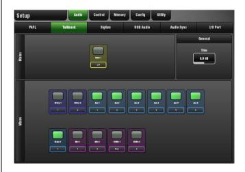
Use this page to assign Talkback to one or more of the Mix outputs. Touch a mix button to assign it On or Off.
