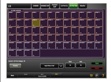
**Patching Outputs** - Touch an output to highlight it. Use the lower part of the screen to select the GLD signal to assign to that output. Open the menu to scroll through and select from the available sources. Choose the source number using the Start box and screen rotary.
