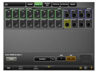
AR84 Expander AudioRack connected to the AR2412 EXPANDER Port – 8 Mic/Line inputs and 4 XLR Line outputs.
