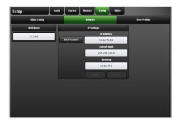
Some functions of the GLD can be controlled using TCP/IP messages via the Network port. The GLD TCP/IP protocol document can be downloaded from <a href="https://www.allen-heath.com">www.allen-heath.com</a>
