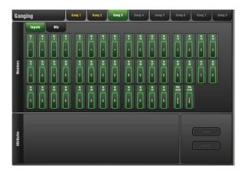
A **Gang** links all or a selection of processing and routing parameters for two or more channels or mixes of the same type. For example, gang two mono input channels to use with a stereo keyboard. The channels or mixes in a Gang are known as 'Members'. The parameters are known as 'Attributes'.
