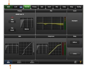
**Active Mix** – Displays the Name and Colour for the Mix currently selected using a fader strip Mix key is displayed at the bottom left of the screen. When the Main (LR) mix is active the status bar simply displays "Main".
