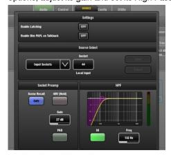
**Enable Latching** – The default Talk switch operation is momentary (press and hold while talking). Turn this option on for latching operation (press to turn Talk on, press again to turn Talk off). Latched operation is useful when you are using a switched microphone for talkback.
