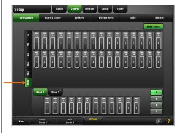
Each fader strip control can be assigned to transmit a custom MIDI message. This is ideal for controlling audio within a Digital Audio Workstation (DAW), a slave mixer, or parameters on external equipment such as effects devices. MIDI Strips can be named and coloured. They are stored within Scenes and can be made Safe from Scene recall.
